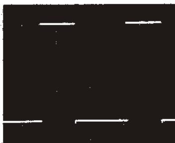
FIG. 12.7. Preset potentiometers correctly adjusted
